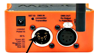
When a DMX cable from your lighting console is inserted into this port, the SHoW Baby automatically switches itself to be a Transmitter.
